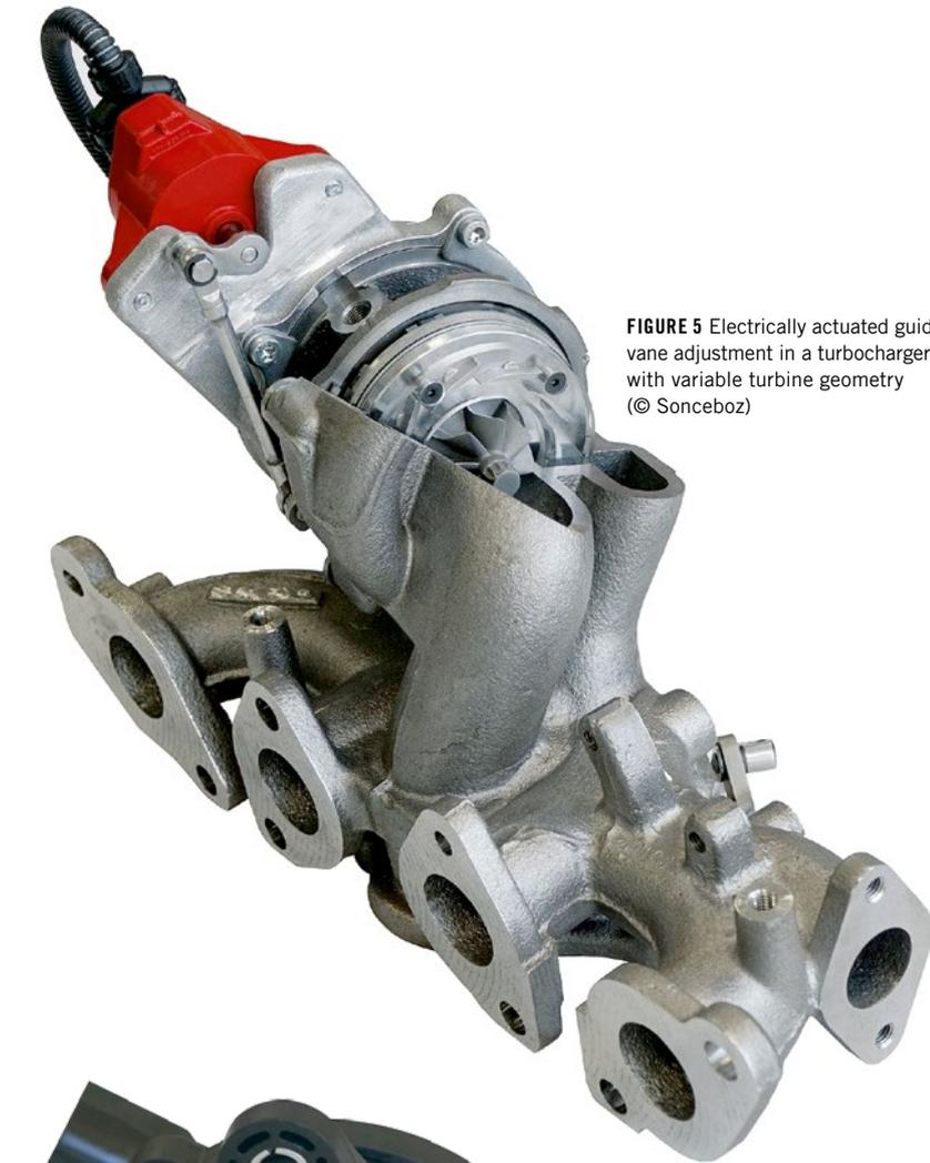
**FIGURE 5** Electrically actuated guide vane adjustment in a turbocharger with variable turbine geometry (© Sonceboz)
